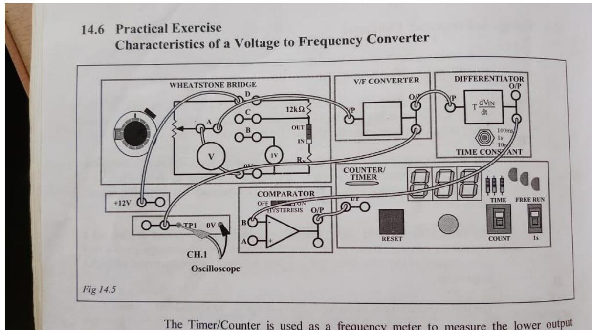
The timer/Counter is used as a frequency meter to measure the lower output frequencies, within its range. The differentiator and comparator are pulse shaping circuits to enable the V/F Converter output to trigger the Timer/Counter.
